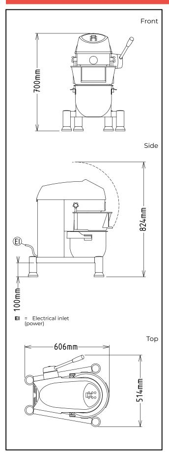
Electric Supply voltage: 380-415 V/3 ph/50 Hz Electrical power, max: 0.5 kW **Total Watts:** 0.5 kW Capacity: Performance (up to): 3.5 kg/Cycle Capacity: 10 litres Key Information: External dimensions, Width: 454 mm External dimensions, 606 mm Depth: External dimensions, Height: 700 mm **Shipping weight:** 57 kg Net weight (kg): 45 **Cold water paste:** 3.5 kg with Spiral hook
